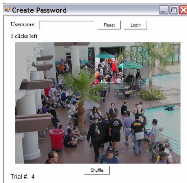
Figure 2: Screenshot of the viewport-CCP Create Password interface persuading users to choose a click-point within the highlighted area ( viewport ). (Pool image from PD Photo 2007)
