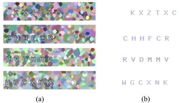
Figure 6. BotBlock CAPTCHA (a) sample challenges (b) challenge text extracted by our automatic program. Note: images in (a) and (b) provide just the same level of security.
