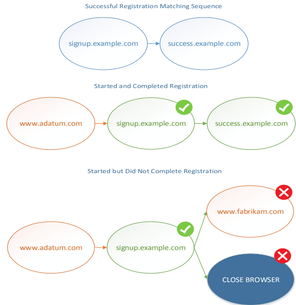
Figure 1: Registration URL sequence matching. Sequences of websites users visited in a session are compared against the known URL sequence for registering an account with the provider. The matching algorithm determines if: (1) the registration process was initiated; (2) the registration process was initiated and finished.
